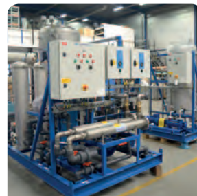
Fully integrated cold water module including disinfection and filtration
